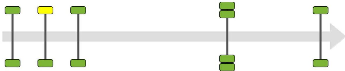
Result of the "Tyre Anomaly and Classification System" (TACS™) on the Highway Rotterdam-Breda where single tyres are being classified as "suspects".
