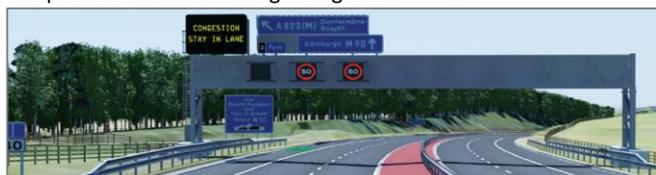
The Intelligent Transport System will allow variable mandatory speed limits to be applied so that vehicle speeds can be managed
